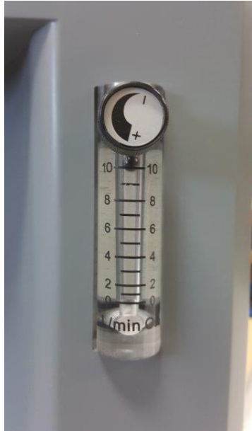
Air unit flow rate adjustment knob
