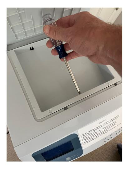
There are two interior filters, they're both towards the front of the air unit, one on the left and one on the right. Reach in and unscrew the top of the filter (the filter housing only turns about 10 degrees and can then be lifted out.
