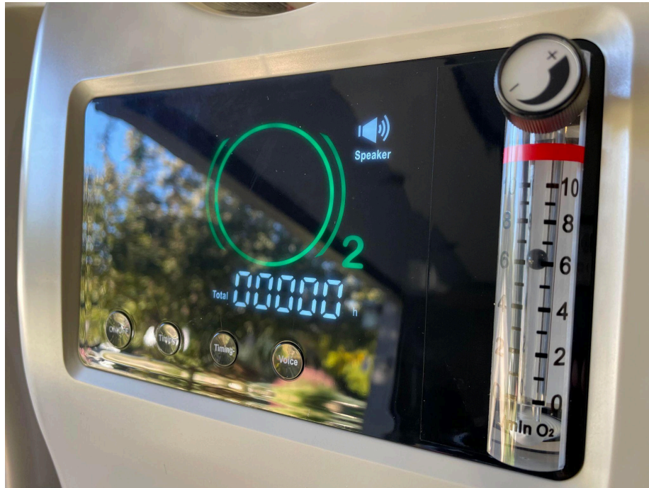
Air unit flow rate adjustment knob
